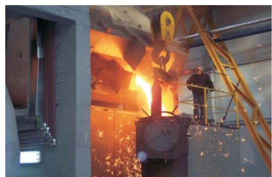
The analysis of each melt is adjusted to the prescribed specifications. A final analysis immediately before pouring ensures the exact composition requirements for each casting. Finally, different ladle treatments are applied to obtain complex metallurgical reactions, a prerequisite for good metal quality and a solid base for the demanding properties of our wide range of materials.
